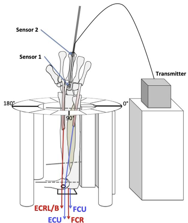
**FIGURE 1:** Experimental setup and positioning of sensors. Each above-elbow specimen was mounted onto a custom-designed testing frame with 1.8-mm-diameter K-wires drilled through the radius and ulna to maintain the neutral forearm rotation. One sensor each was fixed at the dorsal surface of the capitate and the third metacarpal head. Two sensors were aligned in parallel to the third metacarpal shaft. Both sensors were fixed to the bone using nylon tubes and plastic cable ties.
