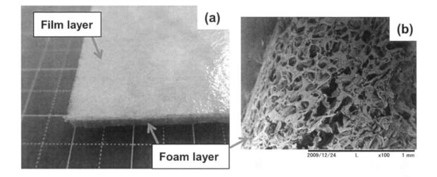
Figure 2. (a) Photograph of the bilayer gelatin sealing sheet and (b) SEM image of the foam layer
