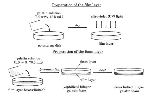
Figure 1. Preparation of gelatin sealing sheet
