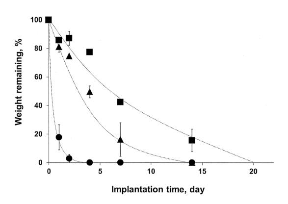
Figure 3. *In vivo* degradation of crosslinked gelatin sealing sheet with different thermal treatment time at 140°C under high vacuum. Treatment time: circle = 2 h, triangle = 3 h, and square = 4 h. Error bars indicate the standard error.
